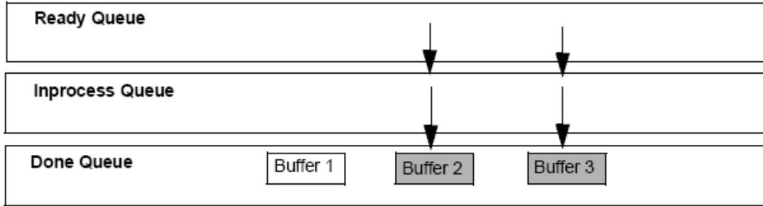
If you transferred data from an in-process queue to a new buffer using **DaFlushFromBufferInprocess**, the new buffer is put on the done queue for your application to process. When the buffer on the in-process queue finishes being filled, this buffer is also put on the done queue; the buffer contains only the samples that were not previously transferred.
