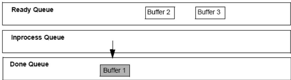
Then, the driver moves Buffer 2 from the ready queue to the inprocess queue and starts filling it with data. When Buffer 2 is filled, Buffer 2 is moved to the done queue and another DA\_WM\_BUFFER\_DONE message is generated.
