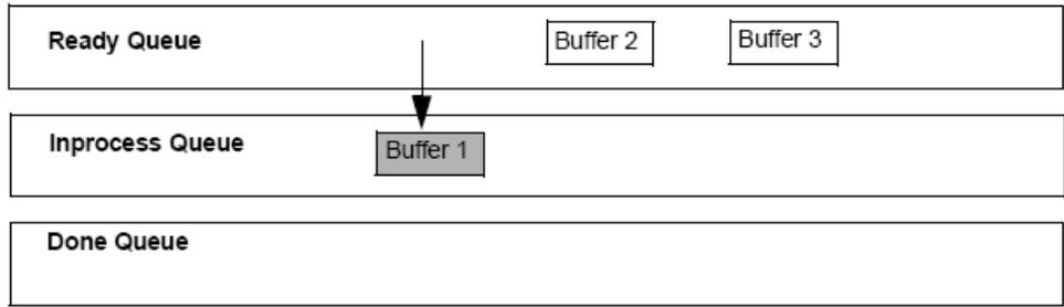
If you want to transfer data from a partially-filled buffer, you can use the **DaFlushFromBufferInprocess** function to transfer data from the buffer on an in-process queue to a buffer you create, if this capability is supported. Typically, you would use this function when your data acquisition operation is running slowly.
