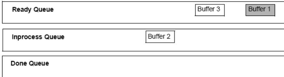
When the data acquisition operation is finished, use the **DaFlushBuffers** function to transfer any data buffers left on the subsystem's ready queue to the done queue.
