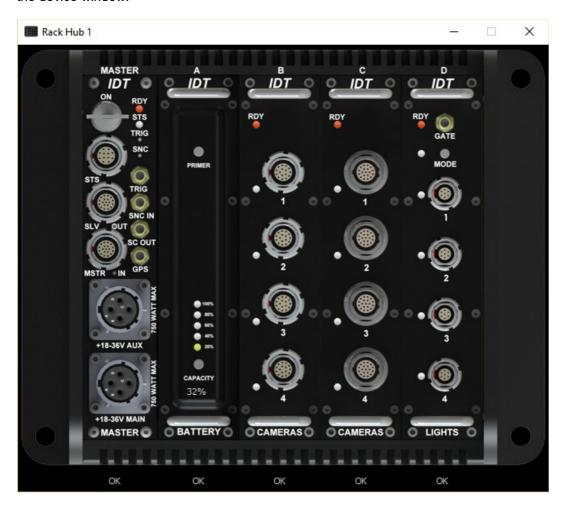
As shown in the illustration above, the 5-slot High G Rack Hub system has MASTER slot and four open slots to be configured with the following available modules (left to right):
