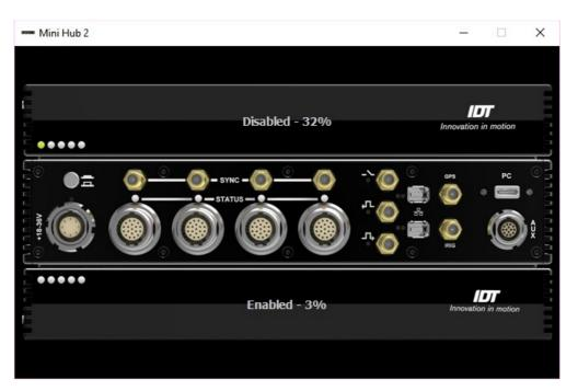
The device includes a master module with support for four cameras and it may include top or bottom battery modules.
