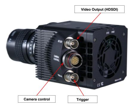
The back panel of Os series is the same with the only difference being the HDSDI connector.
