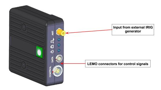
The IRIG flash device is an external box that can be connected to the Y cameras via the external 8-pin and 4-pin control LEMO connectors. The device can be easily hooked to the camera. It is provided with a connector for the IRIG generator and it is fully compatible with the Motion Studio software.
