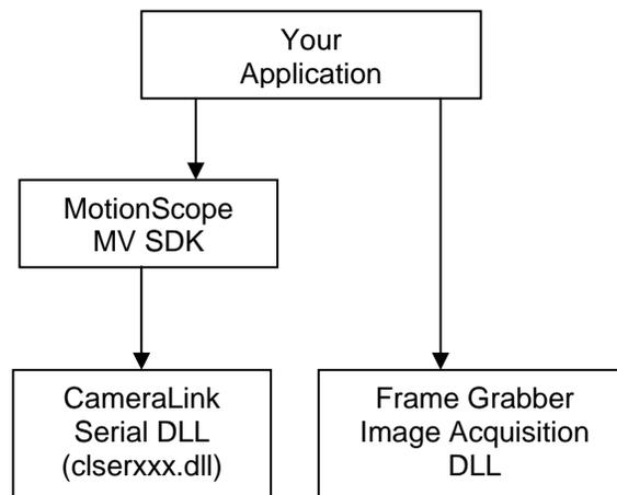
As an option, the user can implement the source code to send commands to the camera via the serial port. The Include subdirectory contains some example C++ files that show how to do it (please refer to the Serial Command Protocol chapter).
