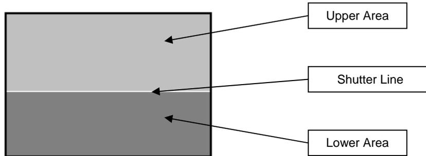
The current value of the shutter line position is returned with a call to `MVGetParameter` with the argument `MVP_SHUTTER_LINE`. The parameter is read-only. If the shutter line is not present and the image does not need correction, the `MVGetParameter` routine returns `MV_E_NO_LINE`.
