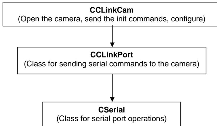
The user should provide routines from the base serial port operations (Open, Close, Read, Write, Flush, Get-Baud-Rates and Set-Baud-Rate). The code will be included in the CSerial class.
